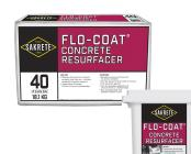
Sakrete® Flo-Coat® Concrete Resurfacer is a polymer modified concrete resurfacing material requiring only the addition of clean potable water. For resurfacing concrete substrates. Can be applied in a flowable consistency using a squeegee, in a stiffer consistency using a trowel or can be sprayed through a hopper gun
